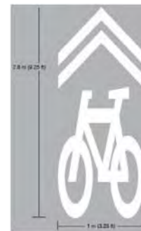
Shared lane marking
